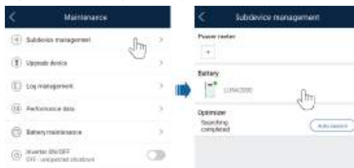
Figure 7-13 Adding a battery
