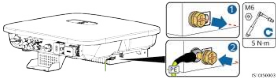
Figure 5-3 Connecting the PE cable
