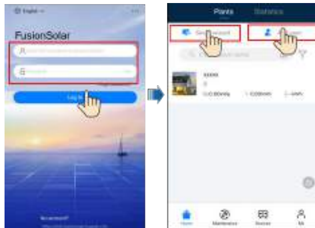
Figure 7-5 Creating a PV plant and a user
